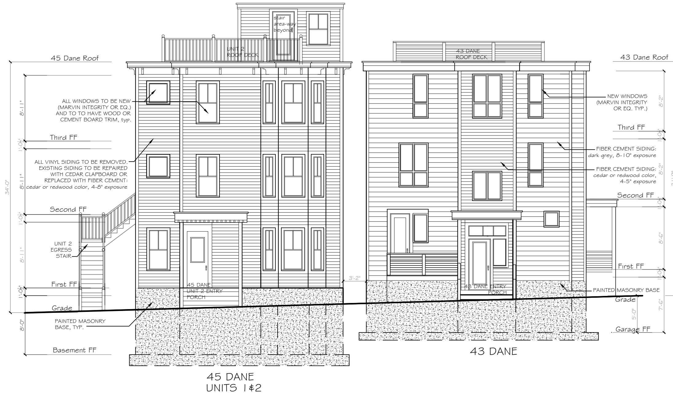
North East / Dane Street Front Elevation
